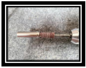
Next, we need to Prep the Shaft Sleeve and install it on the Shaft tip. Prepare the shaft tip the same as any and be sure to Abrade the inside of the sleeve with a Drill sanding sleeve or drill wire brush also will work.
