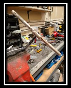
Once drilled and reamed to the Proper Depth you will need to Tap small grooves in the Hosel with a 7/16 Tap small threads and large Threads are just for Good gluing adhesion. The Epoxy I would Use 3M 810 Tan the
