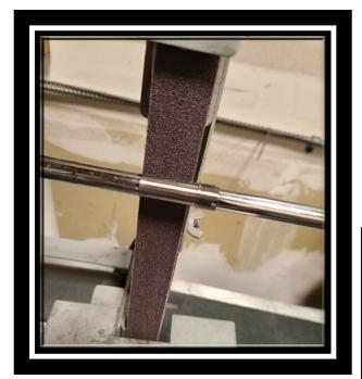
Now glue the sleeve in the prepped hosel and align the open slot to be even with the
