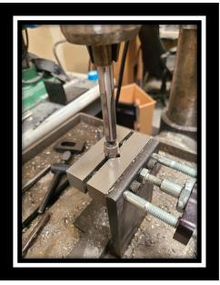
Drill the Iron Hosel with a Drill Bit Smaller than 7/16. This will make the Reaming much easier. Reamer Should Be .440 Solid Carbide Straight Fluted Reamer. Make sure your drill depth is at least 1.210". This will assure that
